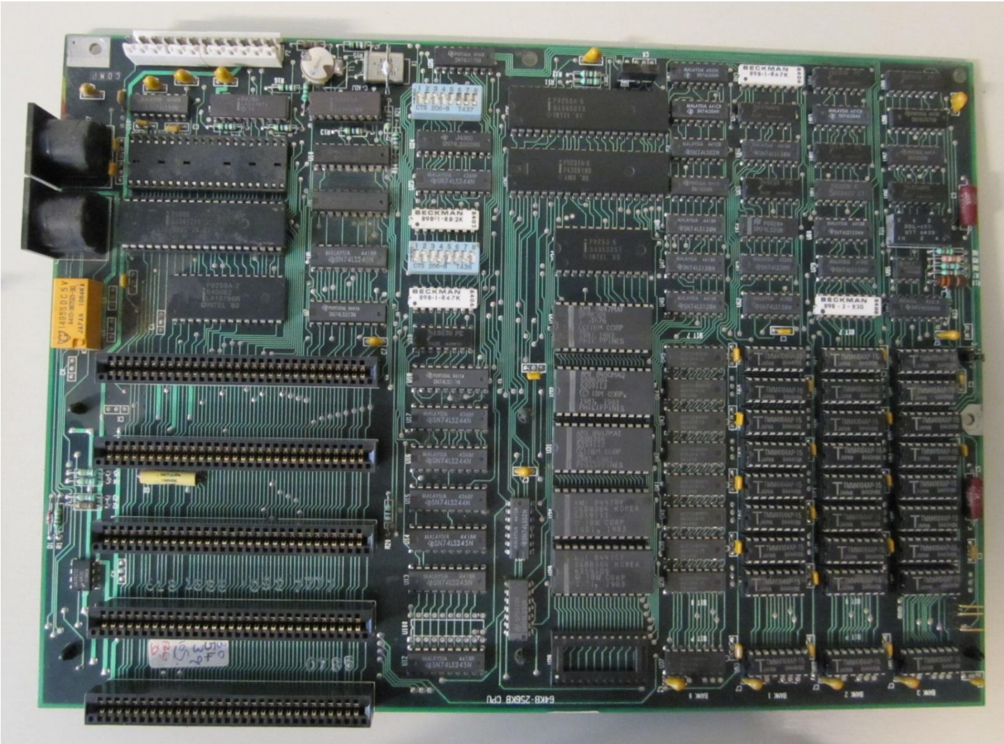
Original IBM PC Motherboard
